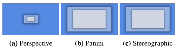
Figure 7: Proportional differences between 110, 140, and 170 degrees of FoV, from inner to outer rectangle, illustrating a disparity between projection methods.
