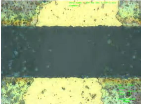
Fig. 15: The green polymer layer on the gold electrode and in the gap of interdigital structure.
