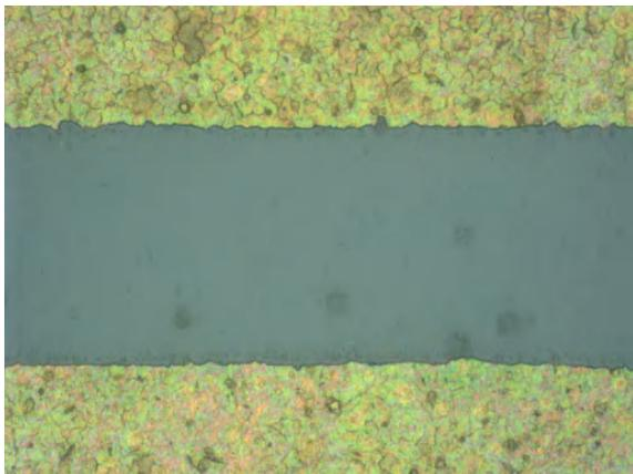
Fig. 4: The created polymer layer for the voltage of 1,5 V and the time of plunge of 60 s.
