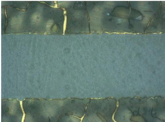
Fig. 12: The created polymer layer for the frequency of 5 Hz, the time of plunge of 60 s and the pulse ratio 2:1.
