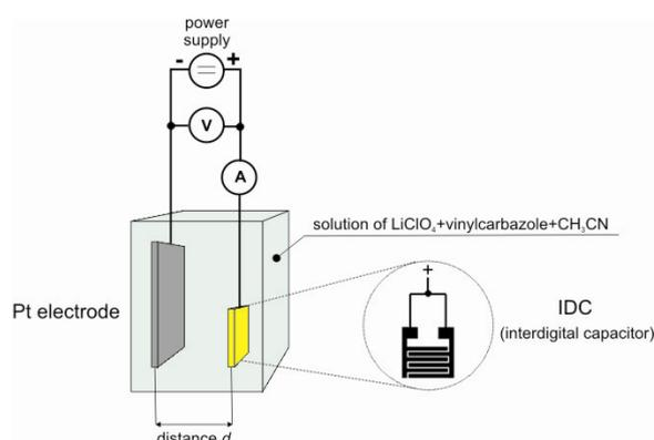
Fig. 1: The basic arrangement for electropolymerization.
