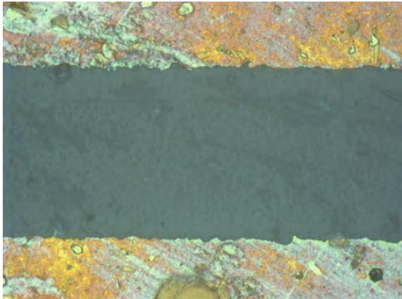
Fig. 11: The created polymer layer for the frequency of 5 Hz, the time of plunge of 60 s and the pulse ratio 1:1.
