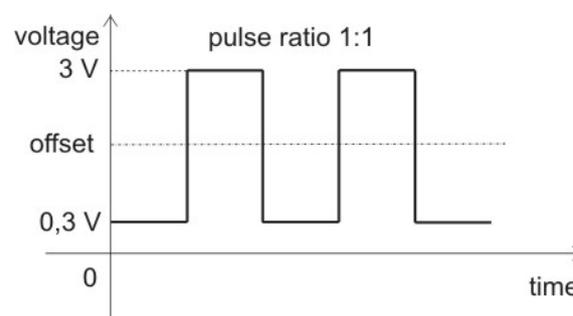
Fig. 10: The output square wave signal from generator with pulse ratio 1:1 and offset 1,6 V.
