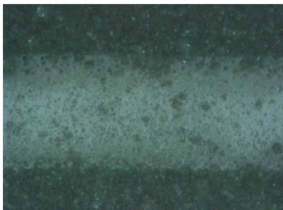
Fig. 8: The created polymer layer for the current of 4 mA and the time of plunge of 60 s.
