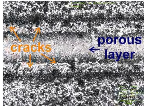
Fig. 17: The created porous polymer layer with cracks.
