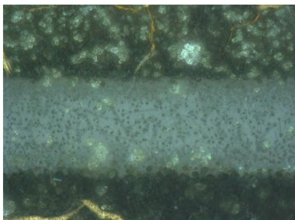
Fig. 9: The created polymer layer for the current of 2 mA and the time of plunge of 180 s.
