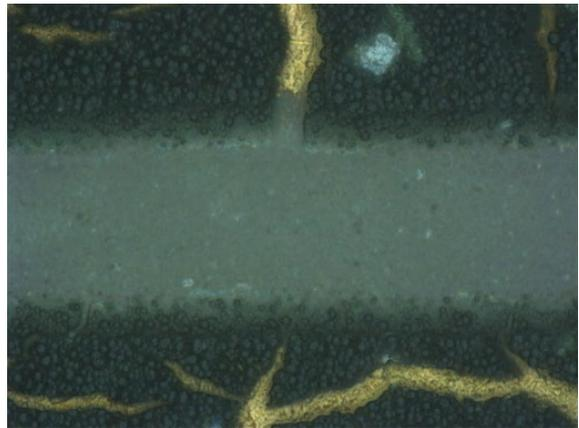
Fig. 6: The created polymer layer for the voltage of 3,5 V and the time of plunge of 60 s.
