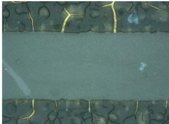
Fig. 14: The created polymer layer for the frequency of 5 Hz, the time of plunge of 60 s and the pulse ratio 8:1.
