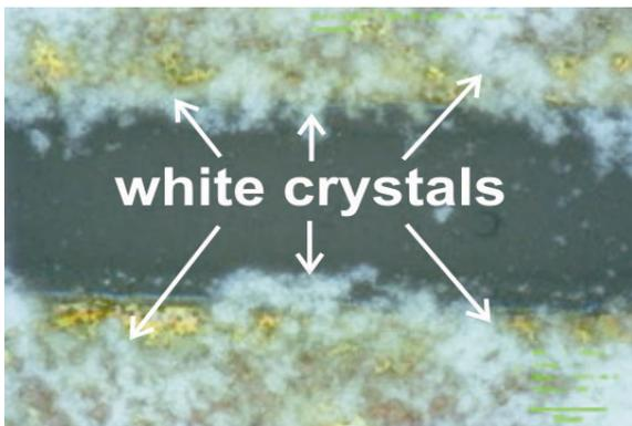
Fig. 16: The white crystals on created polymer layer.
