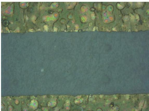
Fig. 13: The created polymer layer for the frequency of 5 Hz, the time of plunge of 60 s and the pulse ratio 3:1.
