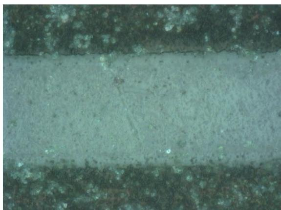
Fig. 7: The created polymer layer for the current of 2 mA and the time of plunge of 60 s.
