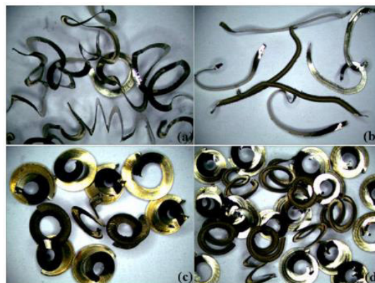
Figure 2.28 Chip forms in AISI 304 milling: (a) dry milling with WC; (b) dry milling with TiN coated WC; (c) MQL millin with WC; (d) MQL milling with TiN coated WC [25]
