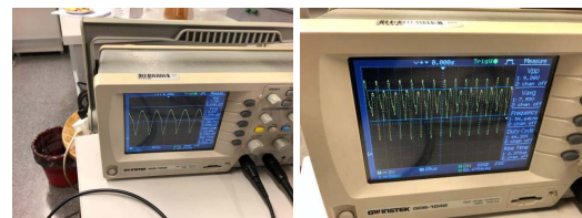
Figure 4. Example of a waveform used in tests. Left: The waveform corresponds to a period one oscillation, see [8]. Right: The waveform corresponds to a period two oscillation (see [8]).
