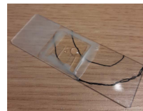
Figure 7. Glass plate with cells as used in experiments. The line draw indicate the approximate position of the capacitor plates.
