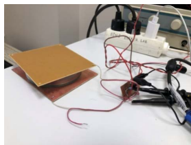
Figure 6. View of the excitation capacitor (on PCB) with the Petri dish inside.
