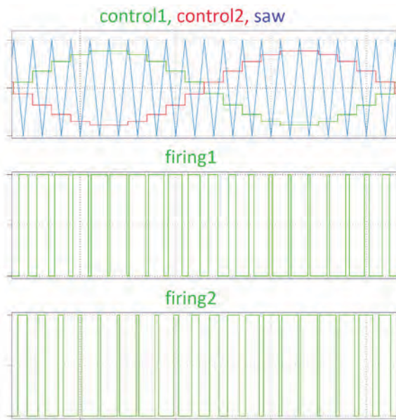
Figure 2. Illustration of signals PWM for H-Bridge cell based on modulation with zero vector alternating
