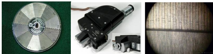
Fig. 3. Components for roughness measurement - comparing a sample card with a real surface
