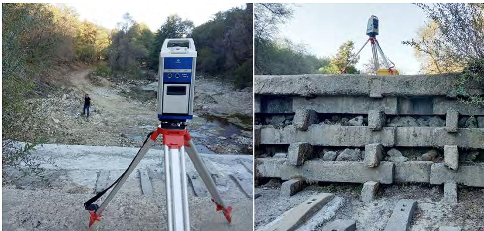
Figure 2. Stonex X300 laser scanner at operation in Damdere debris area
