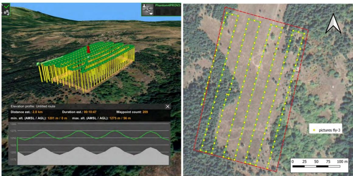
Figure 5. Flight mission FP3: (a) UgCS work screen; (b) Location of the taken images
