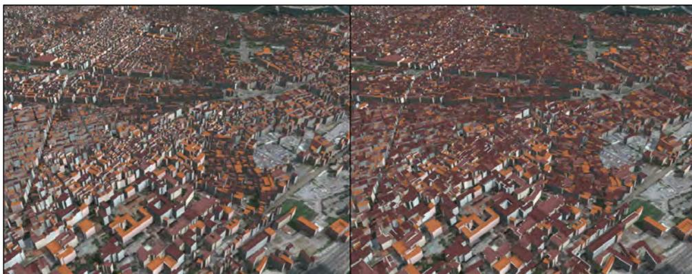
Figure 5. Procedural modeling (left) at basic LOD2 level, advanced LOD2 procedural modeling (right) including roof and facade details.
