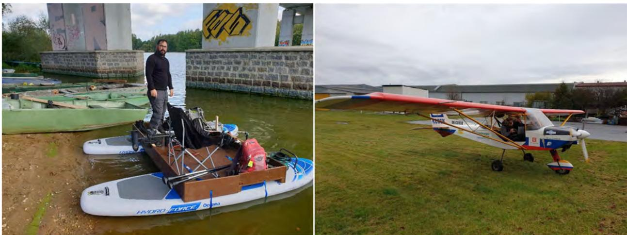
Figure 2 Plattform used for bathymetric survey and small aircraft used for photogrammetrical and LiDAR survey
