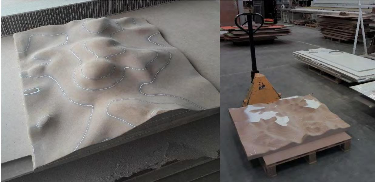
*Figure 11. Prototype 1x1 meter tiles milled into hardboard*
