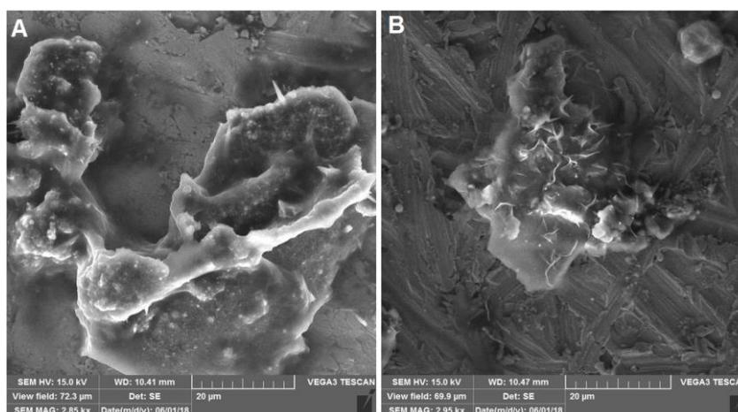
**Fig. 2** SEM images of the FeS particles obtained after evaporation of water (A) and ethanol (B)
