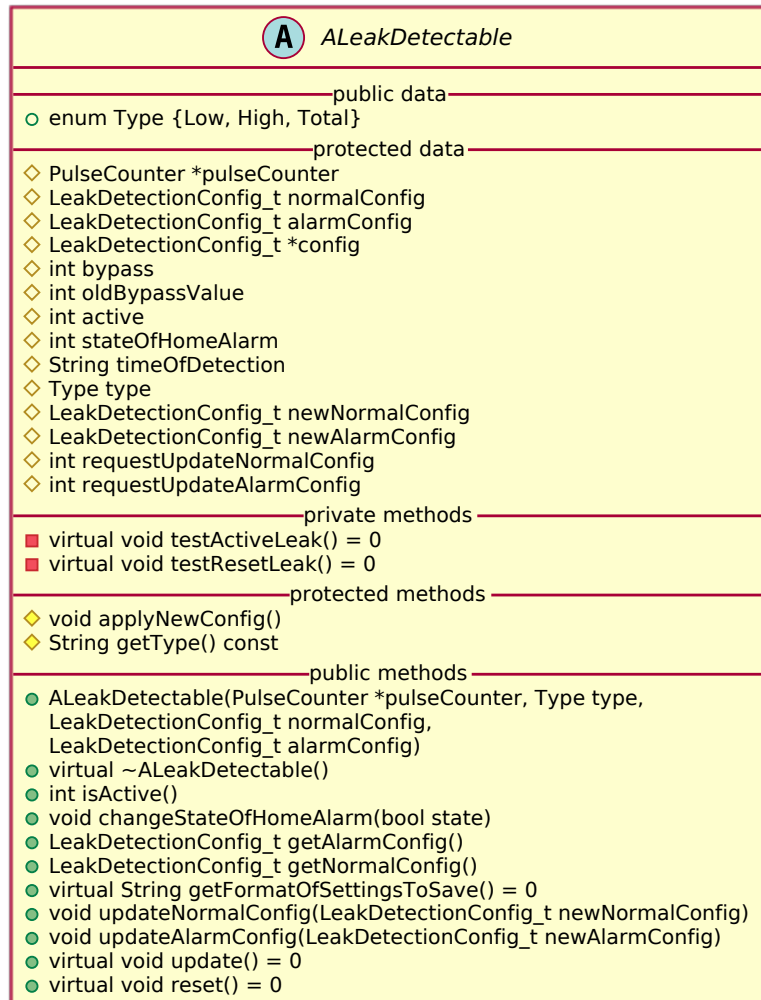
Figure 14.4: UML diagram of abstract class ALeakDetectable
