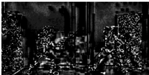
Figure 2. The logarithm of difference between compressed and uncompressed input view of Fencing sequence for high compression. The contrast of the image was increased to increase the visibility of differences.
