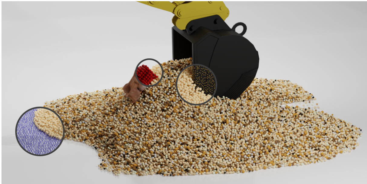
Figure 3: Volume and surface samplings used in a unified simulation framework simulating a granular material and a rigid-body (red) moved by an excavator.
