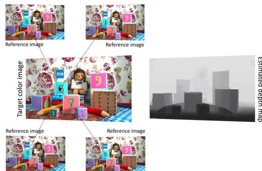
Figure 3: Estimation of depth map using five reference views.
