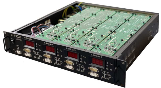
Fig. 9. Universal multi H-bridge converter (SHRack)
