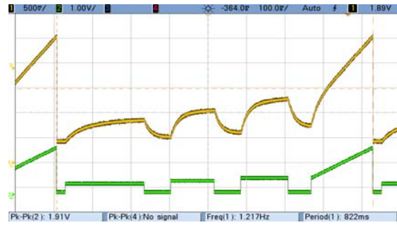
Figure 12. The copy of the oscilloscope screen. VO_2 (top), load (bottom) - simulation by means of electrical circuit
