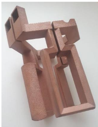
Fig. 2. Example of an inductor produced by additive manufacturing (Courtesy: SMS Elotherm GmbH)
