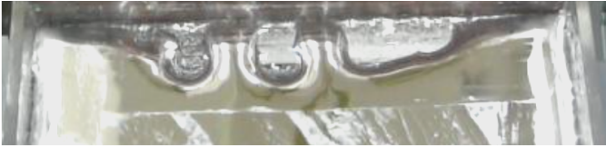
Fig. 2. Oxidized galinstan free surface shape in experiments; melt thickness 4 mm, current 1500 A, frequency 5330 Hz.
