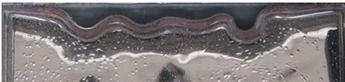
Fig. 4. Non-oxidized galinstan free surface shape in experiments; melt thickness 11 mm, current 2585 A, frequency 4270 Hz.
