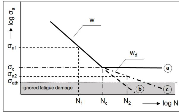
Fig. 3. Boundary conditions for calculating cumulative fatigue damage:
