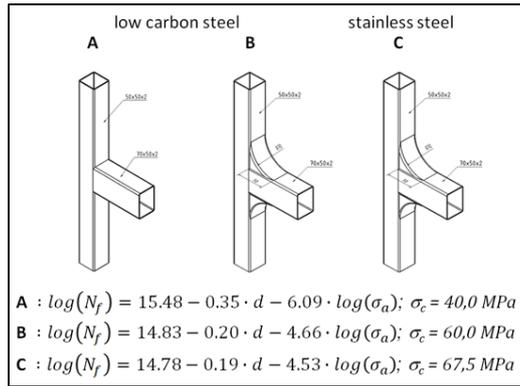
Fig. 4. Bodywork structural nodes and S-N curves
