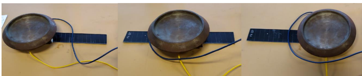
Figure 33 Measuring with a longitudinal probe
