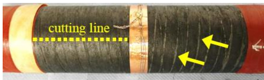
Figure 19 Round profile specimen for simulation of OCP erosion [13]
