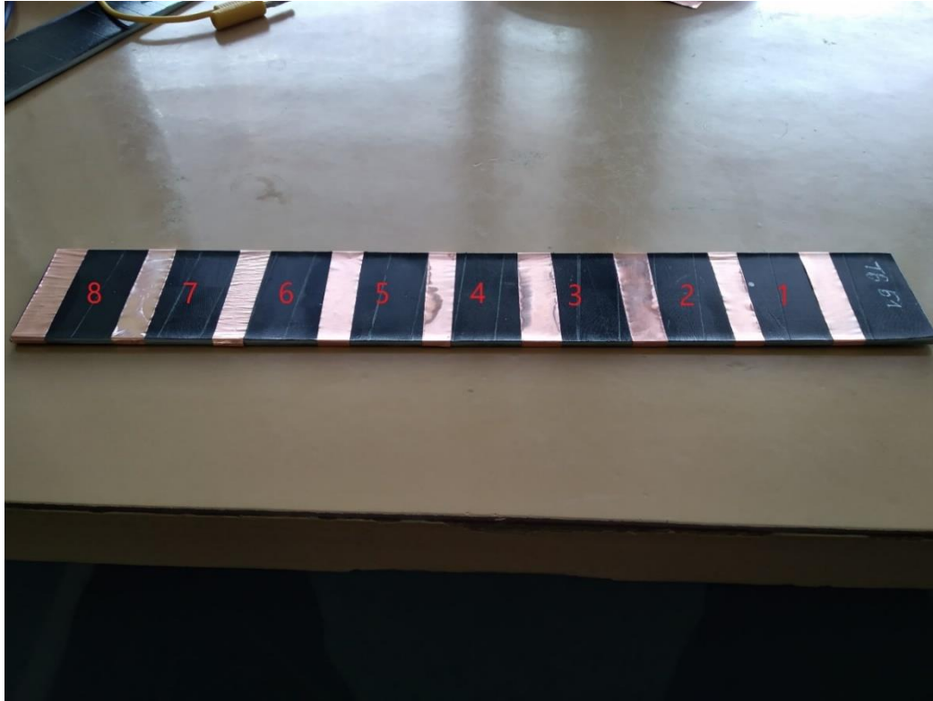
Figure 38 Copper straps configuration on samples
