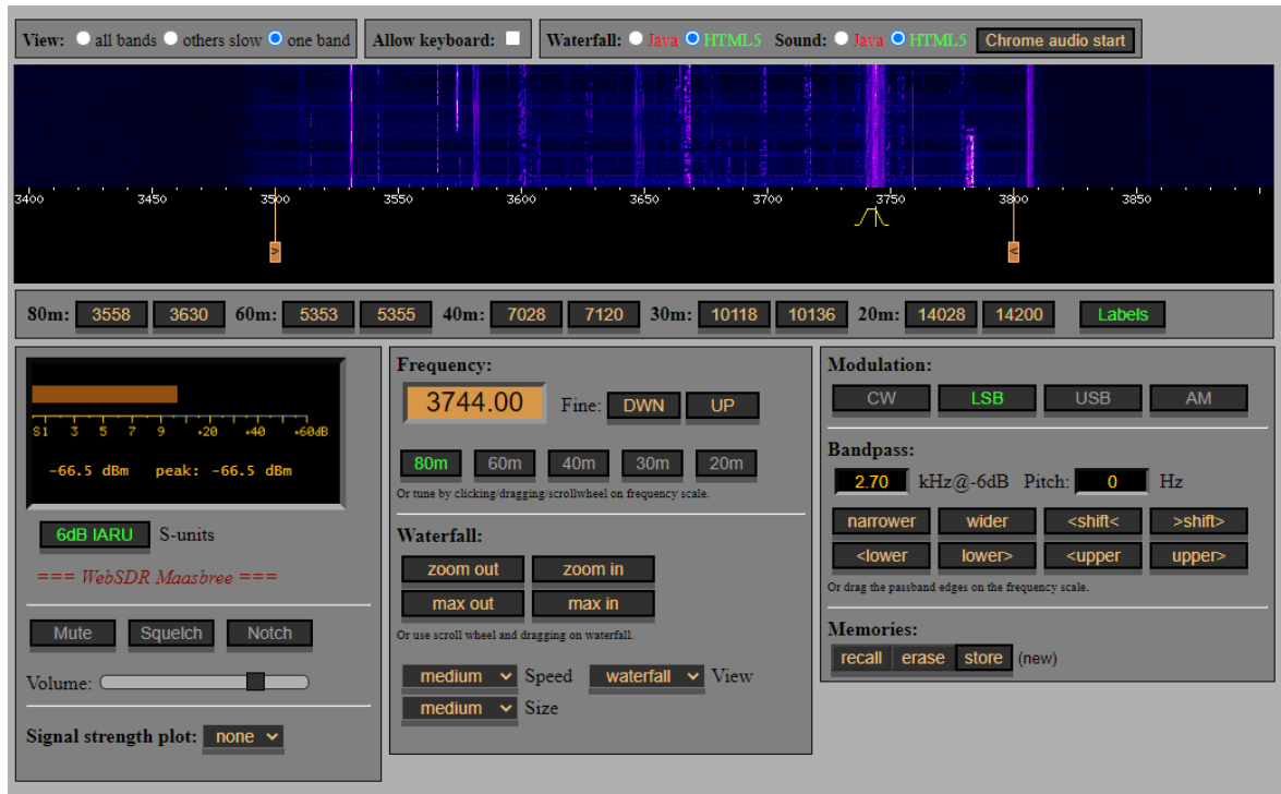
Figure 7: web SDR software configuration[8]
