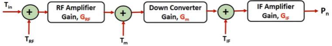
Figure 13:Equivalent receiver where each device is replaced by a single noise source [20]
