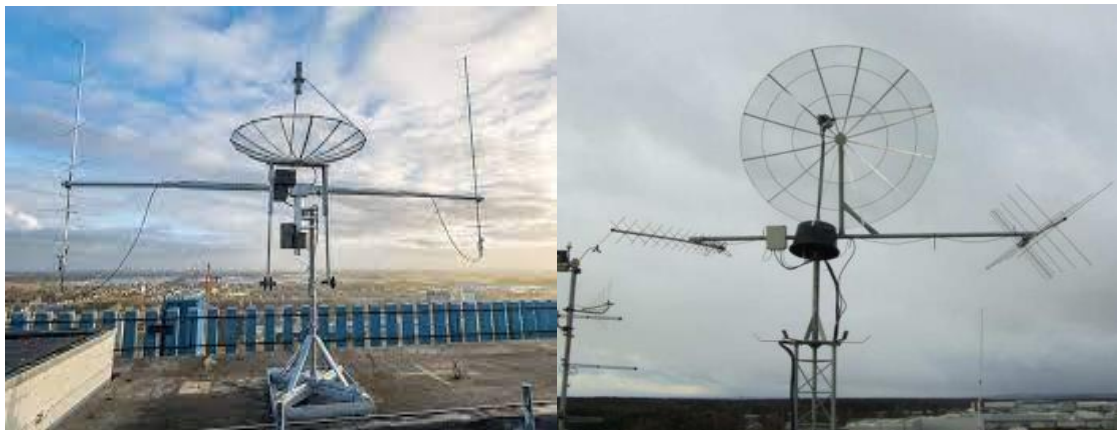
Figure 3: Ground station with rotator[4]
