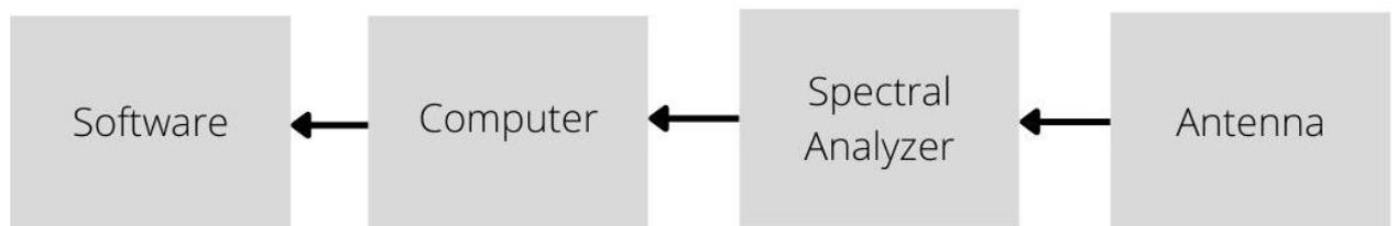
Pic.13 Schematic diagram of measurements
