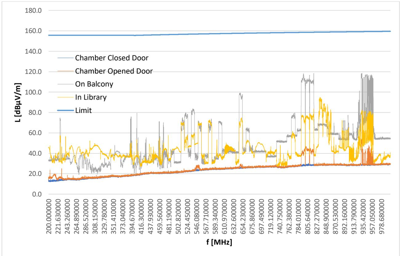
Fig.6 Result for 200 MHz-1 GHz, vertical
