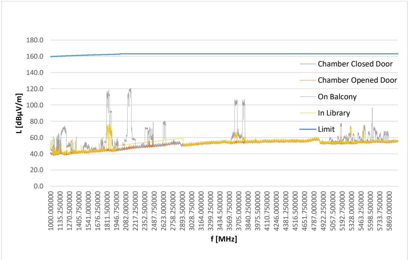
Fig.8 Result for 1-6GHz, vertical
