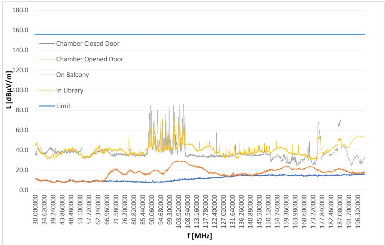
Fig.4 Result for 30-200 MHz, vertical
