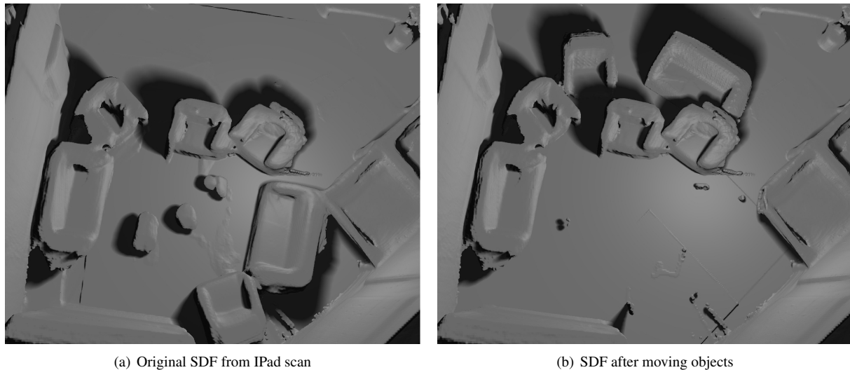
Figure 9: Manipulation of an SDF using the move operator. The SDF was reconstructed from an RGB-D scan obtained by an iPad.
