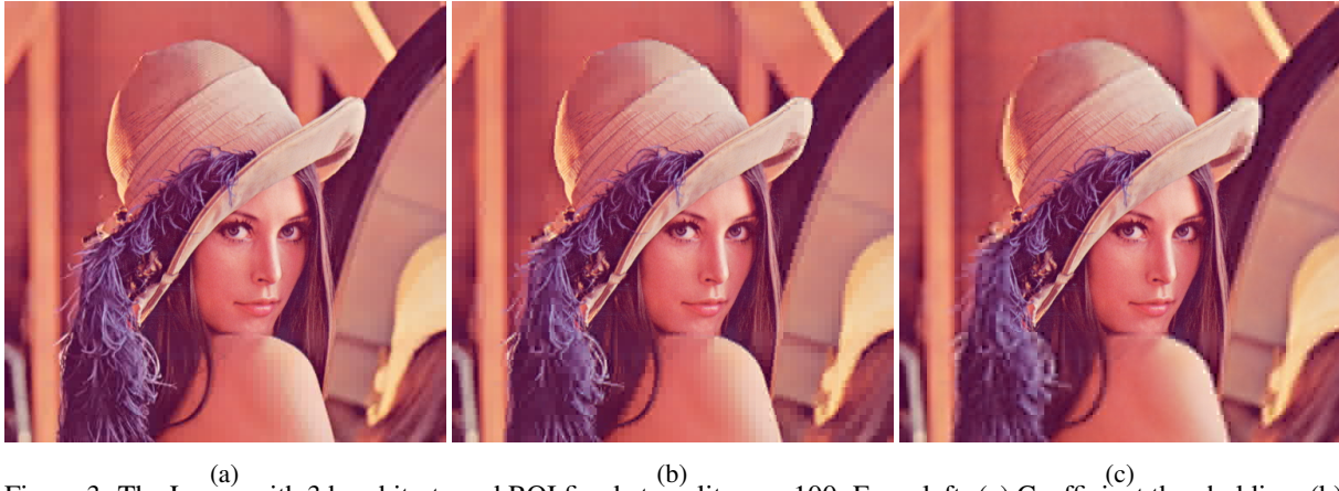
Figure 3: The Lenna with 3 bpp bitrate and ROI fixed at quality q = 100 . From left: (a) Coefficient thresholding, (b) Quantized coefficient thresholding, and (c) Cutting of coefficients.
