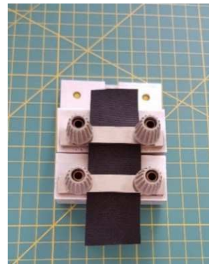
Fig. 5 Electrode system for uncured tapes - surface resistivity measurement
