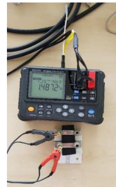
Fig. 6 Measurement with HIOKI RM3548
