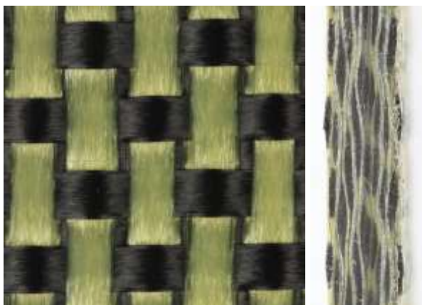
Fig. 1. Detail of hybrid textile composite plate made of 10 layers of plain-weave fabric with carbon and aramid tows and thermoplastic matrix (left – top view ca 10×10 mm, right – side view). Overall thickness is ca 2.5 mm.
