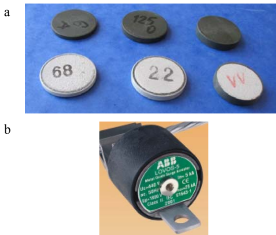
Fig. 3: Varistor structures: a - after being fired (top row) and with a metallized contacts (bottom row); left – 280 V, middle – 440 V, right – 660 V; b - surge arrester with ZnO varistor
