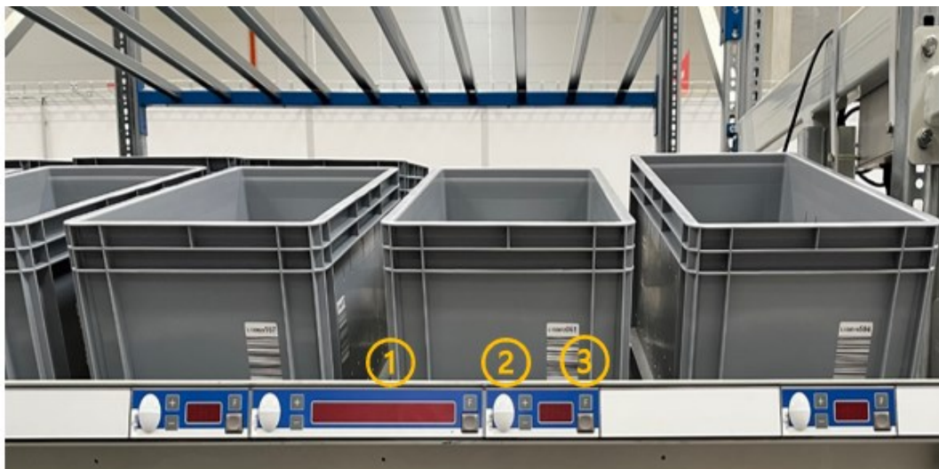
Obr. 16: Sklad se systémem pick by light
