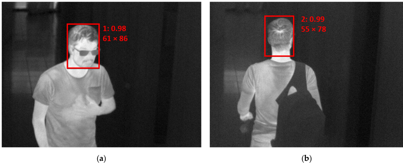
Figure 3. Example of detection by AI: (a) head front; (b) head back (both pictures is author 2).
