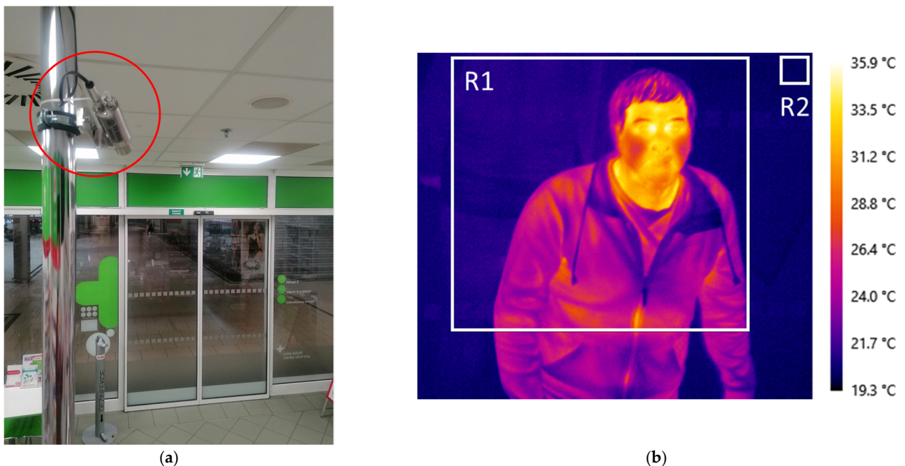
Figure 1. The place of measurement system installation—pharmacy in a shopping center: (a) placement of the IR camera (highlighted in red oval) and its view to the automatic entrance doors; (b) IR image (thermogram) of passing person (author 1).
