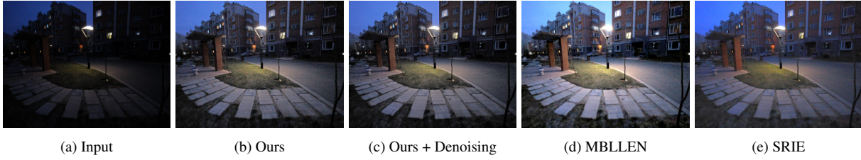
Figure 12: Our result can further be improved by a post-processing denoising operation. Here, we compare our denoised-output (denoising done using FFDNET [58]) with that of MBLEN [34] and SRIE [31].
