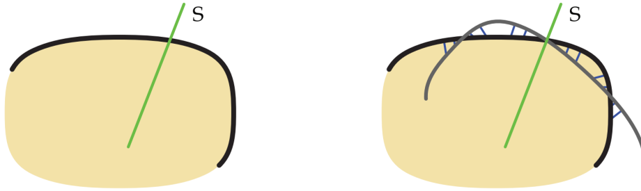
Figure 3.7: Example of the correspondence creation. Left image shows an input surface (the black curve) and a plane in a given iteration of the ICP-like process (the green line S ). Right image shows also the reflection of the original surface over the plane (the grey curve) and the created correspondences (the small blue lines) (figure taken from [29]).
