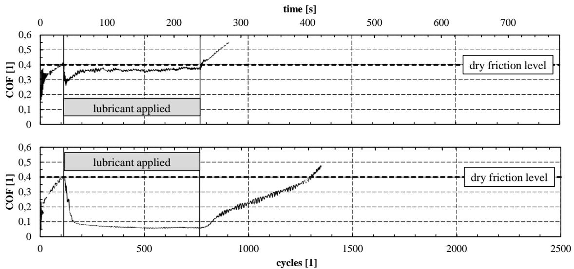
Fig. 1. Measured time histories of COF during twin-disc tests of two different solid lubricants
