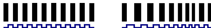
Fig. 3.2 Rectangular signal in case of zero (left) and nonzero (right) torsional vibration.
