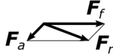
Fig. 1.15 Construction of the resultant magnetic field F_r as a superposition of the armature mmf F_a and field mmf F_f .
