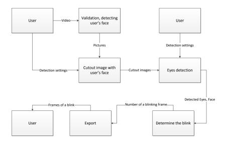
Figure 3.17: Blink Detector - context diagram.
