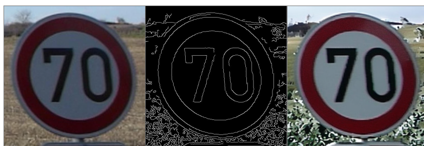
Figure 1: Left: Source image. Middle: Canny edge detector map. Right: Output image from the Stable Diffusion conditioned with the Canny map
