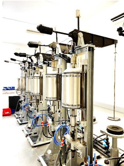
Figure 4-4 Stand lever arm creep machine.
