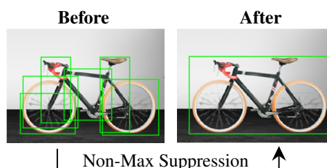
Figure 5: Effect of Non-Max Suppression (NMS). The post-processing technique Non-maximum suppression reduces the number of overlapping bounding boxes.
