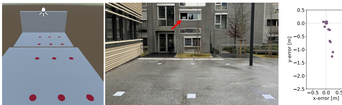
Figure 7: (Left) A simple reconstruction of the test environment in Unity . (Middle) Real-world setup of our test corresponding to the reconstruction. The prototype's position is indicated with a red arrow. (Right) Mean of all deviations from the target location. The error increases with distance to the spotlight due to the cumulative nature of errors in the aiming angle. Note that all targets were still illuminated as the spotlights light cone increased with the distance.
