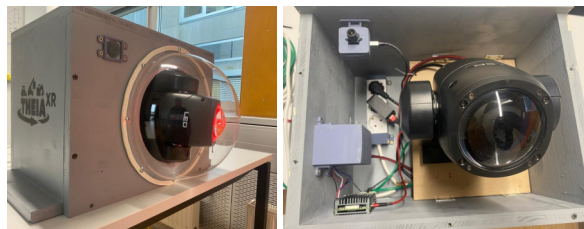
Figure 4: (Left) The assembled prototype in its sealed and finished case. (Right) The prototype without the frontal wood panel and the acrylic half dome.
