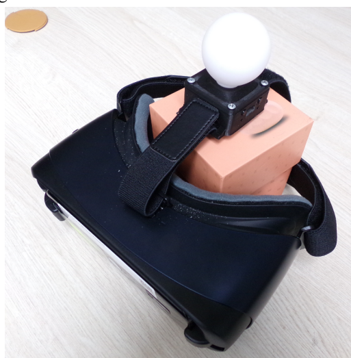
Figure 2. Active marker connected to VR head-mounted display.
