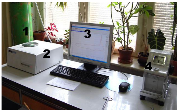
Fig. 3: The DSC Perkin Elmer – 1 gas, 2 DSC, 3 software PYRIS, 4 weighing machine.
