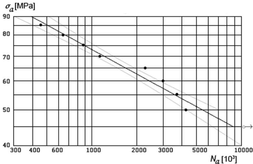
Fig. 3. Wöhler curve for low carbon steel ČSN 41 1523.1 with applied combined pre-stress in normal component  $\sigma_m = 200$  MPa and in shear component  $\tau_m = 133.3$  MPa
