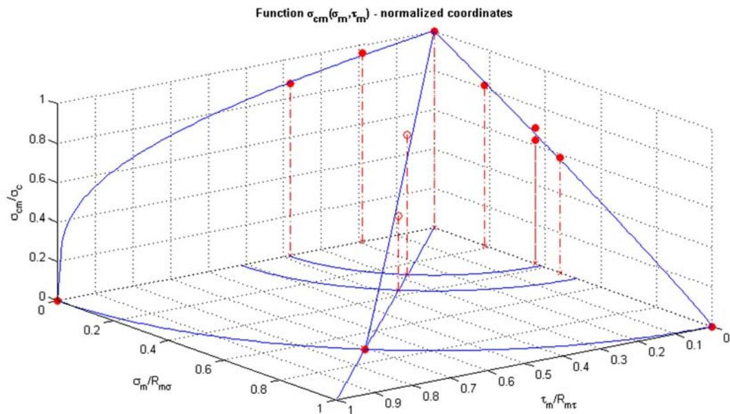
Fig. 4. Haigh diagrams for shear and tensile mean stresses and for their combination in ratio of  $3\sigma_m$  to  $2\tau_m$  that are plotted in normalized coordinates in the three-dimensional graph
