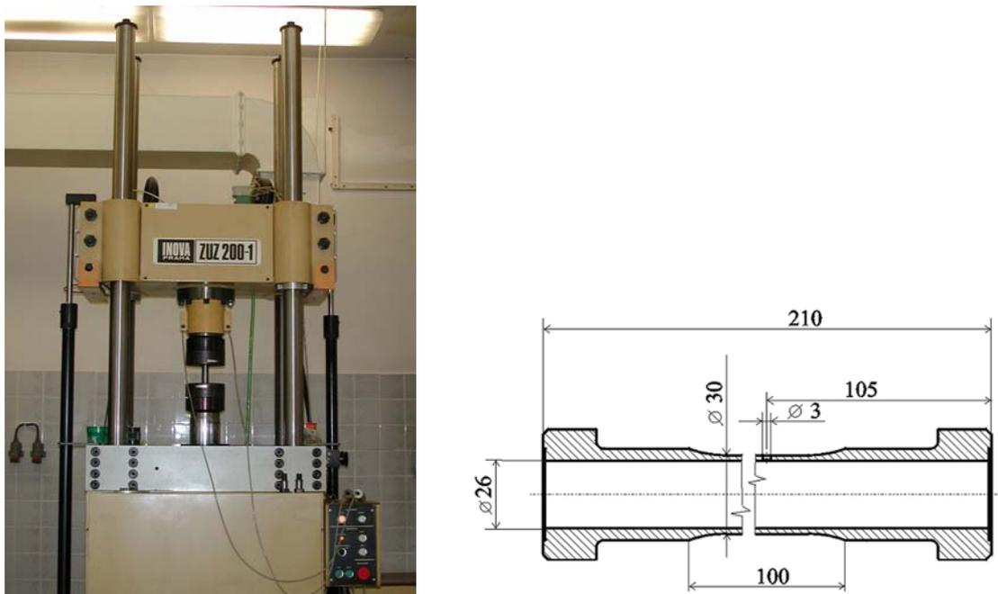
Fig. 1. Servohydraulic fatigue testing machine and dimensions of the specimen
