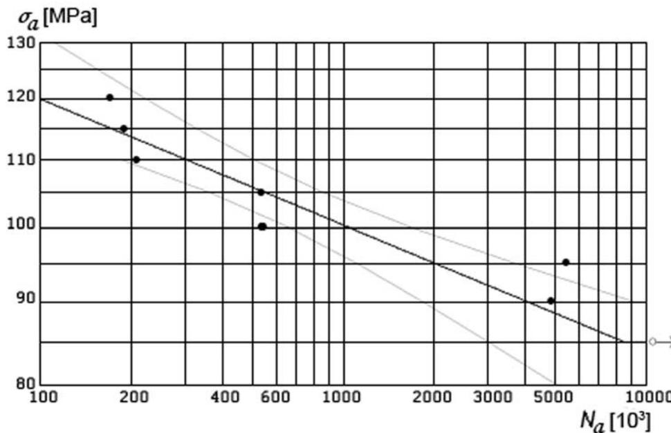
Fig. 2. Wöhler curve for low carbon steel ČSN 41 1523.1 with applied combined pre-stress in normal component  $\sigma_m = 150$  MPa and in shear component  $\tau_m = 100$  MPa
