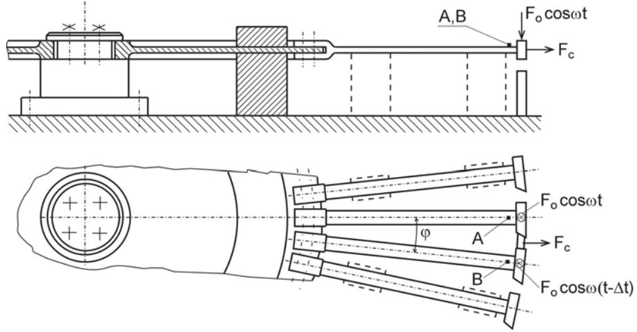
Fig. 2. Measurement of blade couple with inserted friction element
