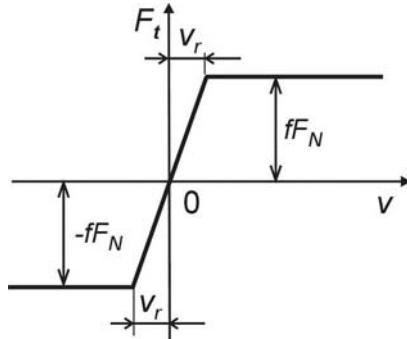
Fig. 4. Modified Coulomb friction characteristics
