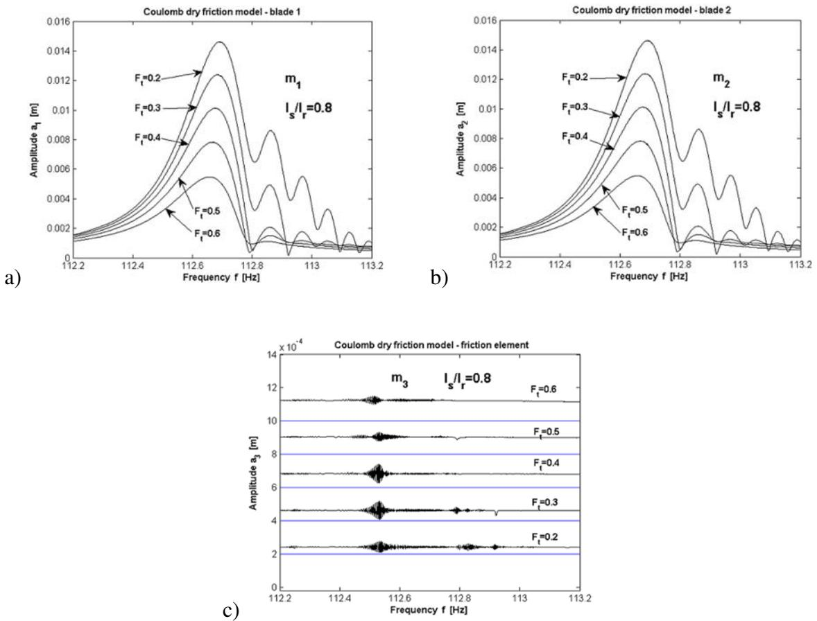
Fig. 13. Influence of different dry friction forces  $F_T = 0.2\text{--}0.6$  at  $l_s/l_r = 0.8$
