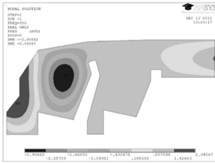
Fig. 5. Acoustic pressure from the finite element analysis. Excitation frequency of  $f = 350$  Hz
