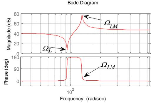
Figure 4: Frequency characteristic of two-mass system.
