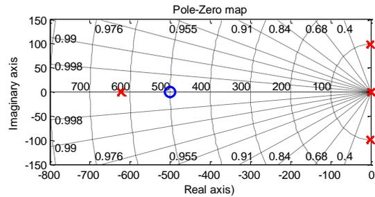
Fig. 7: Distribution of poles and zeros except of remote pole - 2100.
