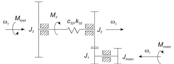
Fig. 2: Principal chart of two-mass system mechanical chain.
