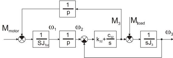
Fig. 3: Model of two-mass system.
