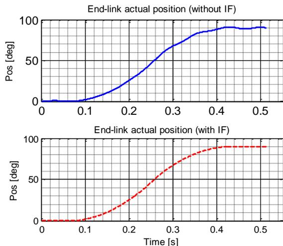
Fig. 8: End-link actual position response with disabled (blue-solid) and enabled (red-dashed) inverse filter vibration compensator.
