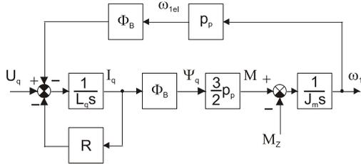
Fig. 1: Model of permanent magnet synchronous motor.
