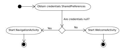
Figure 15.1: Activity diagram of application startup
