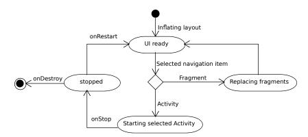
Figure 15.3: Activity diagram of NavigationActivity
