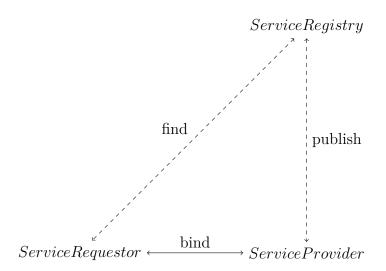
Figure 5.1: Communication diagram between web service elements [3]
