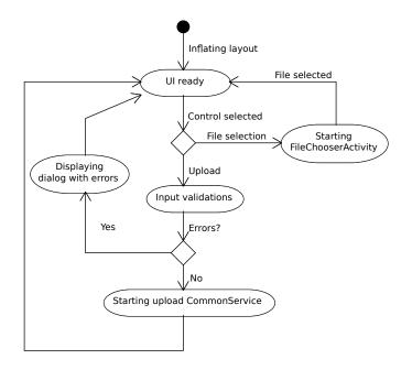
Figure 15.5: Activity diagram of DataFileUploadFragment
