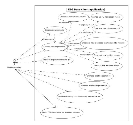
Figure 4.1: EEG Database client application use case diagram
