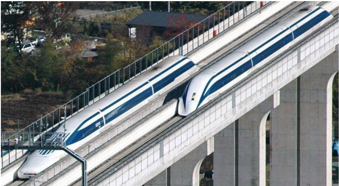
Appendix E: The latest superconducting maglev system MLX01 and older version MLU002 N [19]
